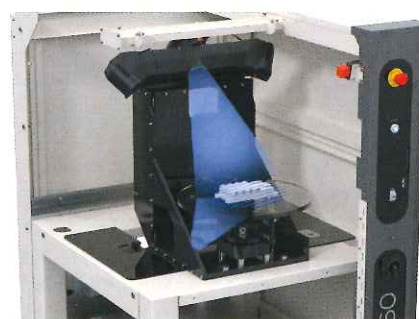
With just one button, the CyberGage360 conducts a highly precise 360-degree 3D scan of complex parts, accurate to 7µm.
