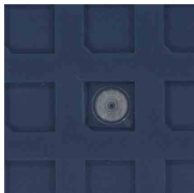
Lens Inspection - Bubble Defect
