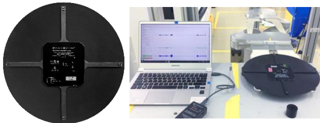
Figure 1 AMS sensor (left) and sensor with associated communications module and laptop computer (right) providing data acquisition and analysis.
