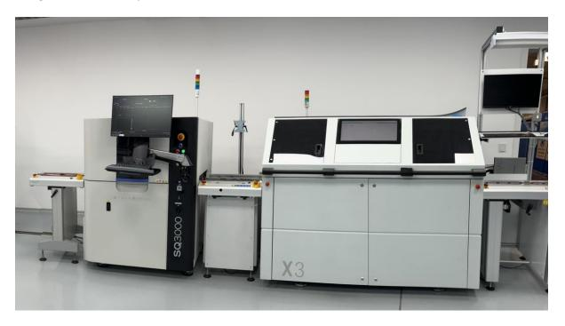
The CyberOptics SQ3000 Multi-Function system, deemed best-in-class, can identify critical defects and measure critical parameters, in order to fix what can be found and control what can be measured. In addition to AOI and SPI applications, highly accurate coordinate measurements can be attained faster than a traditional Coordinate Measurement Machine (CMM) – in seconds, not hours.
