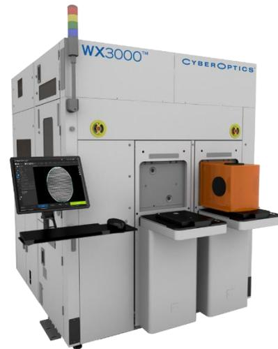
WX3000 systems are designed specifically for various wafer-level and advanced packaging applications including wafer bumps, solder balls and bumps, gold bumps and copper pillars. The systems provide superior measurement and inspection performance for features down to 25-micron, including bump height, coplanarity, diameter and shape, relative location and a variety of other measurements.
