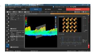
CyberCMM, an extensive suite of CMM tools, provides 100 percent metrology-grade measurement on all critical points much faster than a traditional CMM – seconds, not hours – including coplanarity, distance, height and datum X, Y, to name a few. A fast and easy setup can be performed as compared to a slow, engineering resource-intensive setup that typically requires multiple adjustments with traditional CMMs.
